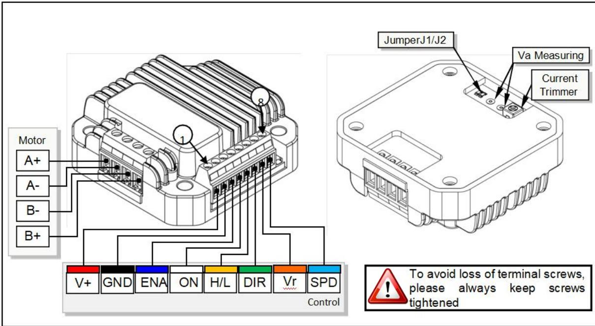
Figure 2:wiring terminal
